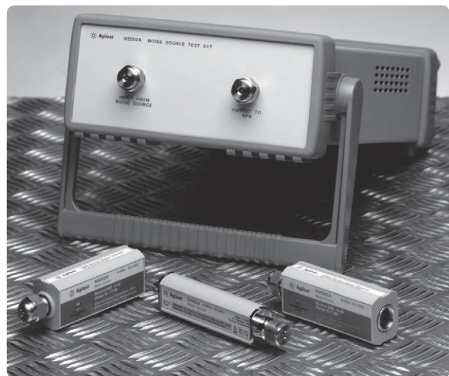
Figure 1. N2002A noise source test set with SNS series and 346 series noise sources
